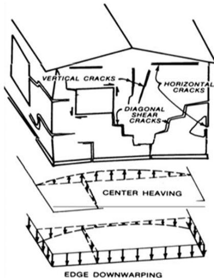
**Figure 1** Cracks patterns on exterior wall resulting from dome heave of foundation soil, [16]
