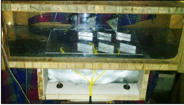
Fig. 1(c) Experimental test section having heated plate with inclined blocks along with equilateral triangles as obstacle
