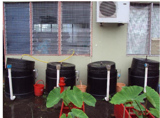
Fig. 1 Photo showing compact biogas plant set up , 500 liters
