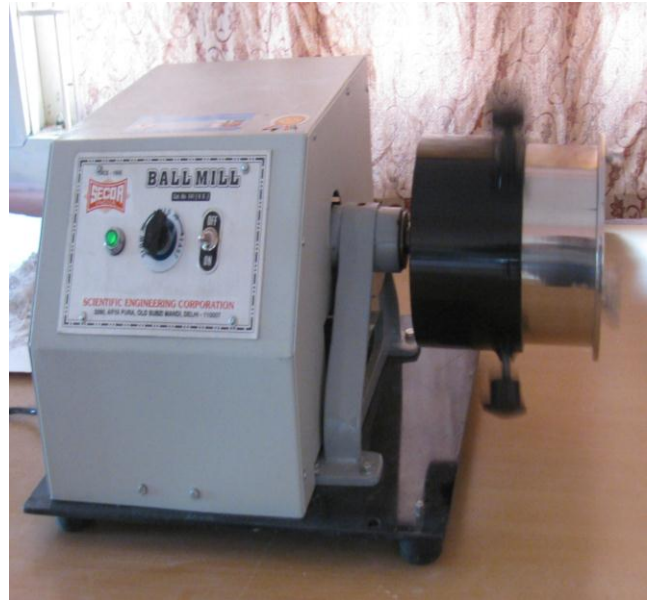
Figure 4 ball mill for the synthesis of nanosilica
