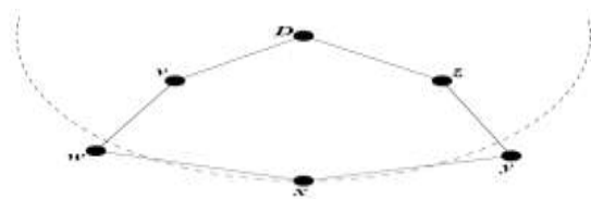
Figure 2 Greedy forwarding failure. x is a local maximum in its geographic proximity to D ; w and y are farther from D .
