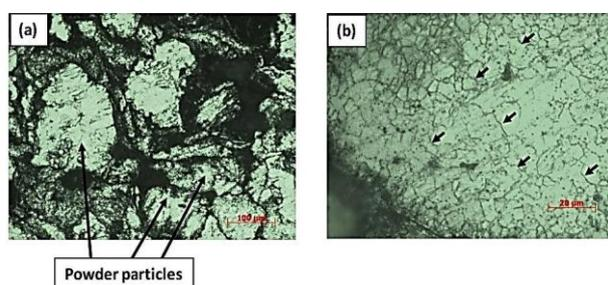
Fig. 6: Optical micrographs of the green compact of mild-steel and 20 wt.% nodular cast-iron powders compressed at 800 MPa obtained at (a) 100X and (b) 500X magnification of optical microscope.
