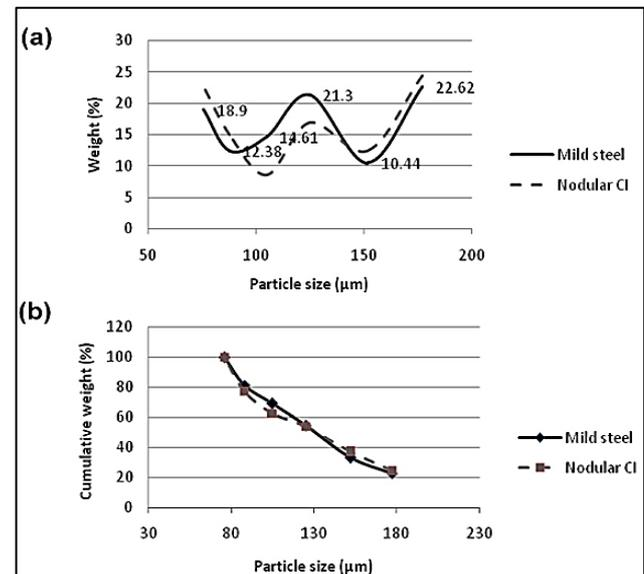
Fig. 5: (a) Particle size-distribution and (b) cumulative particle size-distribution obtained by sieve analysis of mild-steel and nodular cast-iron powders
