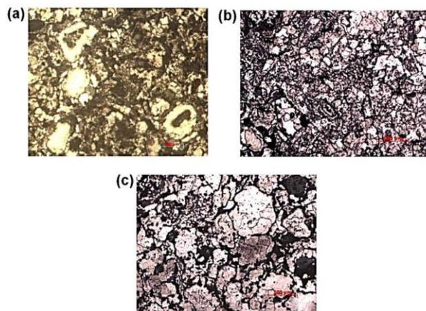
Fig. 7: Micrographs of mild-steel and 20 wt.% nodular cast-iron powder compacts compacted at 800 MPa and sintered at 1100 ± 30 °C for (a) 20 min, (b) 40 min and (c) 60 min. All micrographs are at 100X magnification of the optical microscope.
