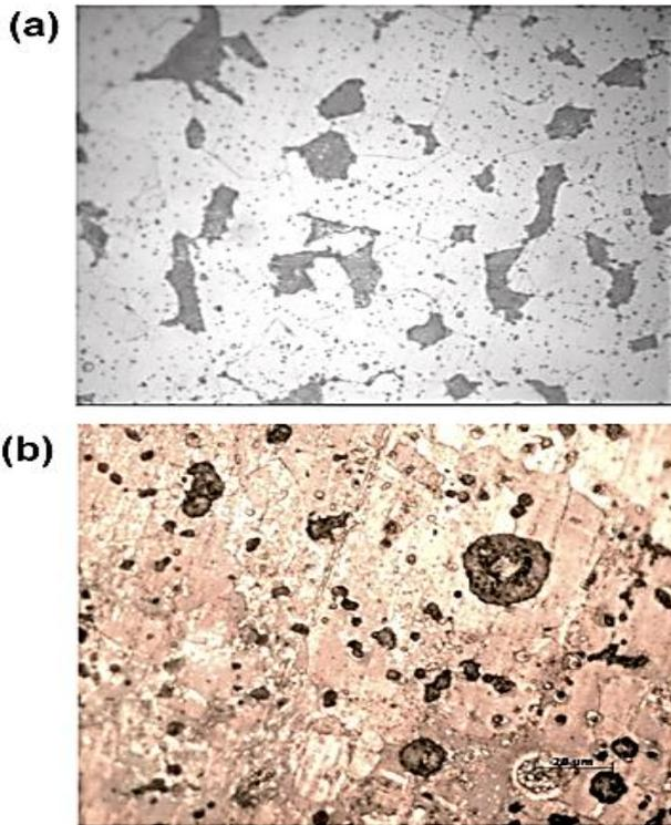
Fig. 3 Optical micrograph of annealed (a) mild-steel and (b) nodular cast-iron
