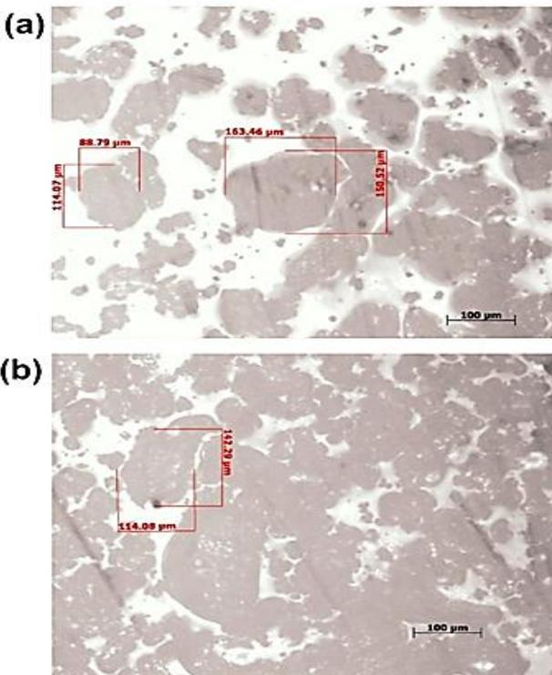
Fig. 4: Micrograph of (a) mild-steel powders and (b) nodular cast-iron powders.
