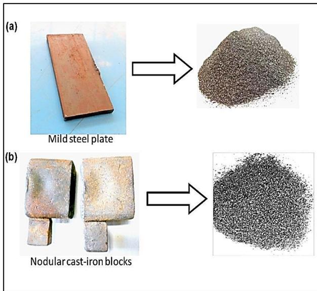
Fig. 1: (a) Mild steel plate into powder and (b) nodular cast iron blocks into powder
