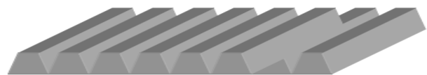
Fig. 1 Wavy plate having horizontal pitches on sharp edges (Trapezoidal wavy bottom plate)
